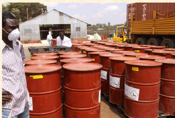
Obsolete pesticides packed in UN approved drums being loaded into the container
